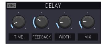
The stereo delay time can either be synchronized to the DAW host or can be set to a fixed frequency value in Hz.
