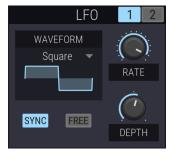
The **LFO** section contains the two LFOs (low frequency oscillator). You can switch between the two by clicking on the tab number.
