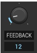
The graphic for each algorithm has a loop drawn around operator D. This indicates that there is a **feedback** loop attached to that operator. The feedback level can be controlled by the feedback knob. This feedback loop modulates operator D with itself.
