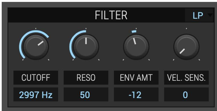
The filter type can be selected in the top right. The filter slope is 24db/oct. You can select between lowpass, highpass or bandpass type.
